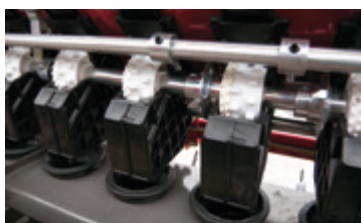
Two-piece integrated metering rollers for cereals and rape
