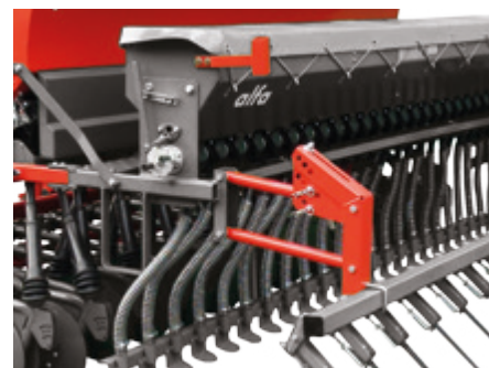
ALFA 180/23/3 (with spreading bar) mounted on POLONEZ seed drill
