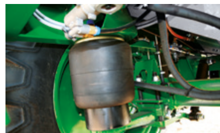
Axle with air shock absorbers improves comfort and prolongs the life of the sprayer.
