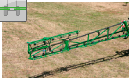
R-SYSTEM, boom working width reduction system: from 28/21 m, 27/21 m, 24/18 m, 21/15 m and 18/12 m. Section of boom is being folded vertically.
