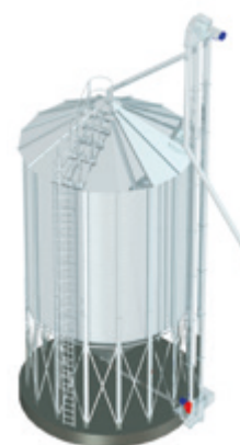
SIDE SURFACE – creates a steel mantle of the silo and consists of specially corrugated sheets made of steel sheet covered with GALFAN which increases durability of the anticorrosion protection. The whole structure is stabilized by a system of vertical reinforcements. Individual elements of the side surface are combined with steel bolts. Simplicity and stability of the structure makes it easier and faster to install.
