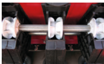
Seeding units for fertilizers (peg wheel)
