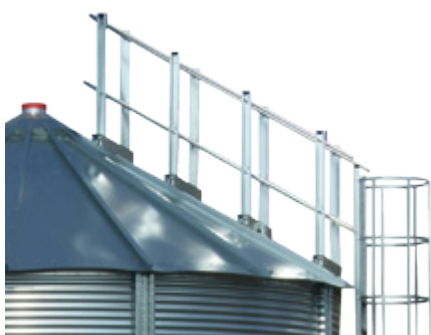
SILo ROOF WITH A GUARD RAIL – cone with a 30 degree angle made of sheet steel covered with GALFAN coating and screwed with bolts
