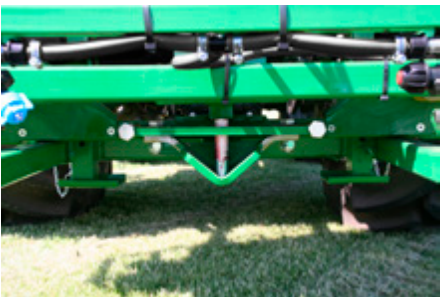
Stabilization interlock allows safe folding and operations with partially unfolded boom.
