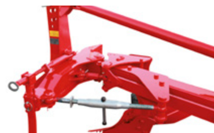
Mechanical adjustment of working width
