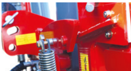
Hydraulic transport blockage integrated with folding cylinder TERIS LH
