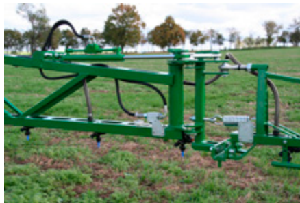
Hinged part of the extreme last section protects the boom against damage during collisions with obstacles.
