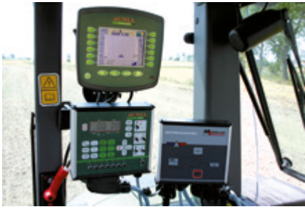
SPRAY computer with NAVI – GPS facilitating spraying and eliminating overlapping.
