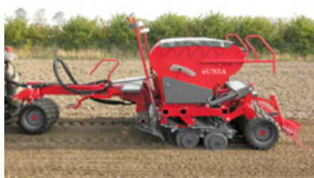
Amber 3000/3 standard version + two disc coulters "V-TECH" 360 mm, side ground following wheels 320 x 64 mm
