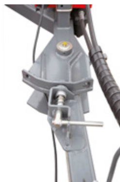
Drawbar – adjustable in three positions. Transport – Operation
