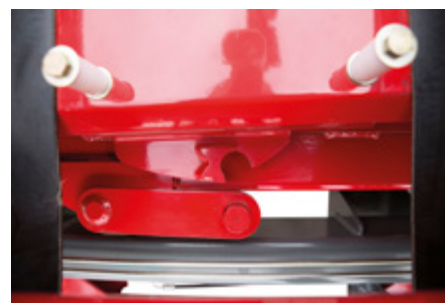
Mechanical turntable lock – stabilizes the turntable when arrival at field or during transport
