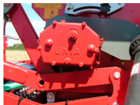
Precise variable gear to adjust the seed dose.
