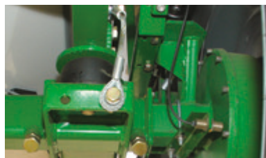
Mechanical shock absorption of axles correct the stability of the beam and durability of the machine considerably.
