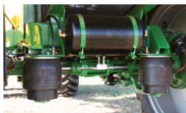
Air shock absorption of axles Air shock absorption improves comfort during fast driving and in the field conditions, it dampers any vibrations transferred to the field boom very effectively.
