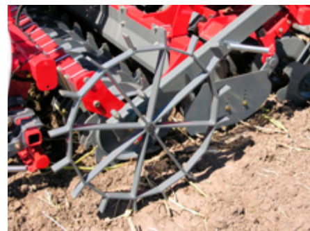
Drive of seeding shaft from the massive spur wheel
