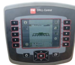
DRILL Control – radar controlled electronic seeding controlled by electric motor
