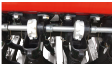
Metering units for fertilizers (volumetric fluted metering unit)
