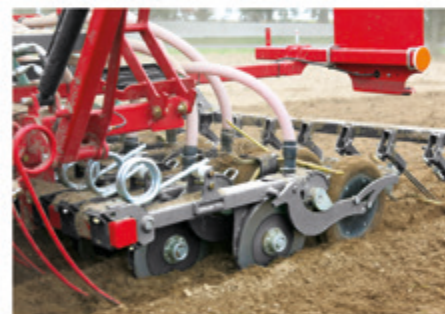
Massive coulter with simple depth control system
