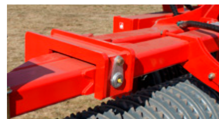
Precise ground-following of particular rollers section based on swinging system.
