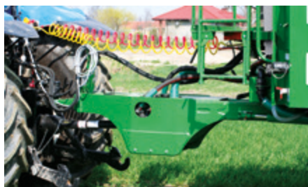
Automatic tracking drawbar facilitates driving in the tractor wheel tracks.
