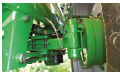
Turnable axle Turnable axle precisely tracks the tractor tracks. Requires UTS computer.
