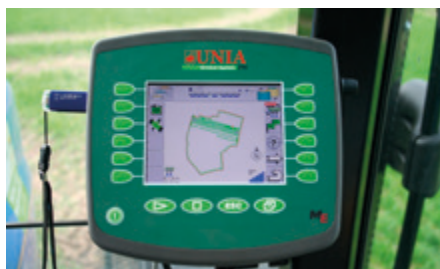
UTS computer with GPS with Track Leader II and Section Control software allows you to take advantage of the precision agriculture.
