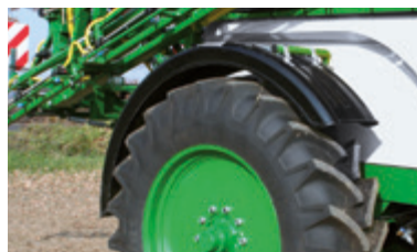
Mudguards Protect the system from dirt liquid beams
