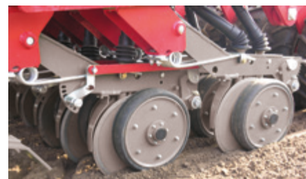
V-TECH coulters with side wheel allows for supreme ground following and place seeds on required depth
