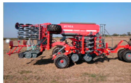
Transport system with pneumatic brake and four transport wheels ensures high stability of the machine for transport.
